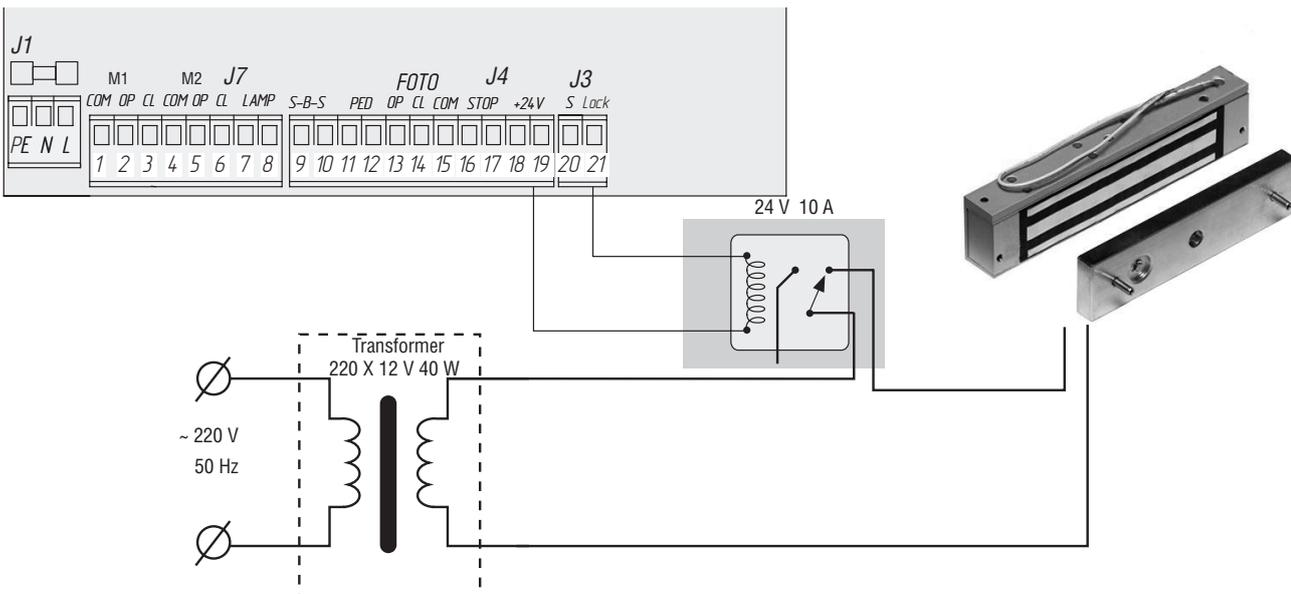
**Connection diagram for electromechanical lock with capacity of up to 3A**
