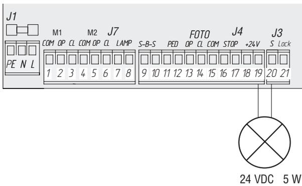
**Connection diagram for auxiliary lighting**
