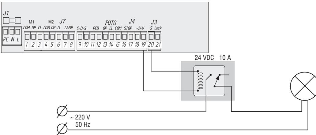
**Connection diagram for auxiliary traffic control signal**
