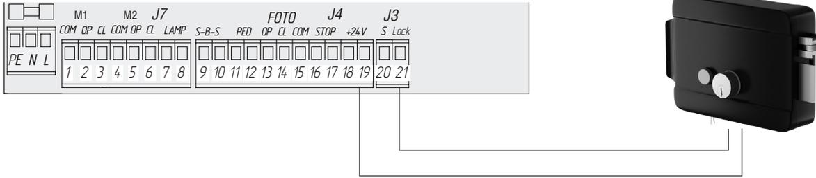
**Connection diagram for electromechanical lock with capacity of more than 3A**
